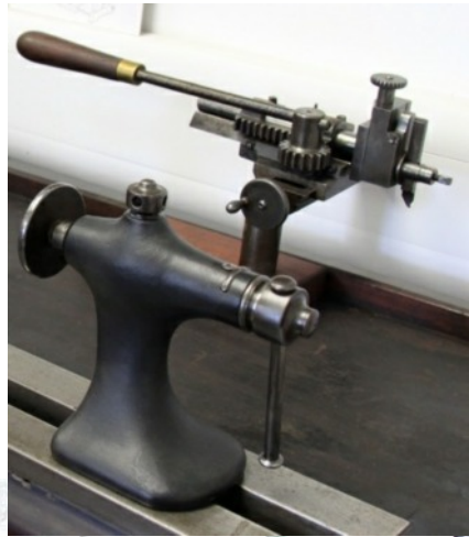
H2083 Telegraph Museum, Porthcurnow (UK) Note the unusual lever operated eccentric cutter
