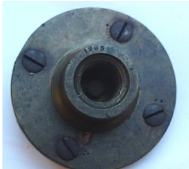
H1983, Drive Plate or Back Plate only (UK)
