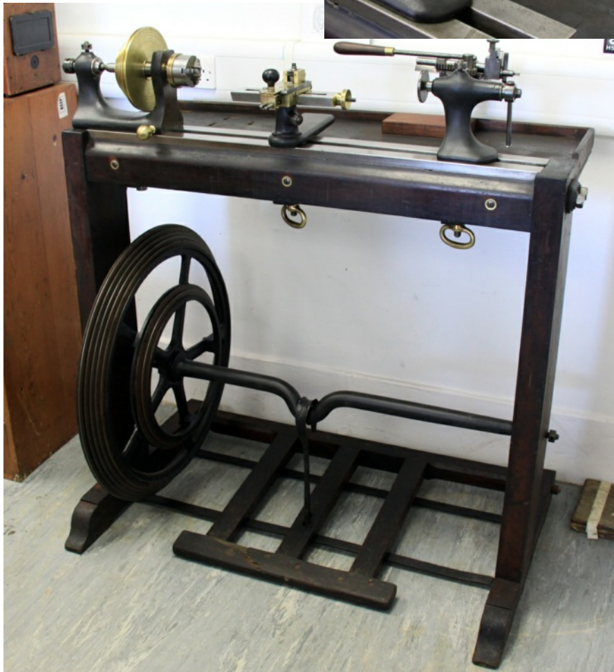
H2083 Telegraph Museum, Porthcurnow (UK) Note the unusual lever operated eccentric cutter
