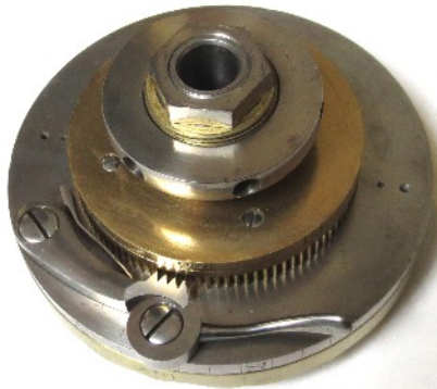
H2245, extra large Rose Chuck with 7" Rosettes, Pumping Apparatus and Automatic Segment Drive (UK)
