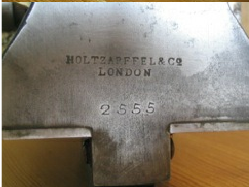
H2555 5" Common Headstock only; later fitted with 180-tooth Worm-wheel and Tangent Screw by Hines of Norwich (Canada)
